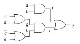
(a) (12 pts) Find a set of test vectors that will test every stuck-at fault. Note: treat  $\bar{c}$  as its own variable, but one that is constrained (in the test vectors) to be the complement of *c*. (e.g. use  $\bar{c}$ 0 to denote  $\bar{c}$  stuck-at-0.)
